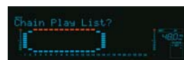
Program Chain Mode: Programs (songs) can be played back in a pre-determined order.
